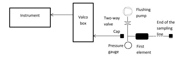
Once the line is plugged, wait until you reach steady state. Then close the valve and turn the pump off and check if the vacuum is stable. If after 20 minutes, there is no change, your line does not present leaks.
