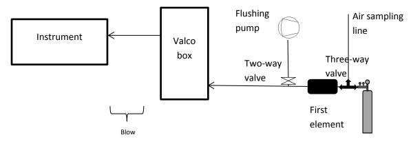
Open the cylinder, then open the pressure regulator in order to match the flow and/or pressure observed for ambient air.
