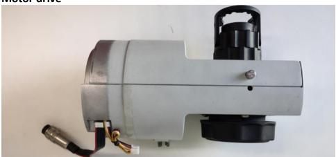
Press and hold down the gray fixing knob and turn the lock counter clockwise. Unscrew the lock from the motor drive.
