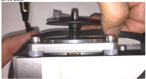
As shown in the picture put the belt in position and rotate the drive disk until the belt glides down correctly.
