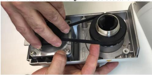
Please check if there is any rubbed residual of the belt in the notch. If necessary, remove the residual with a pointed object.
