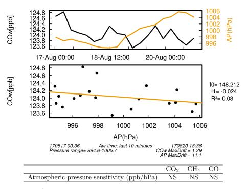
Not significant (NS) if R<sup>2</sup> <0.5 or the absolute value of the slope lower than 1, 0.02 and 0.03 ppb/hPa for CO<sub>2</sub>, CH<sub>4</sub> and CO respectively
