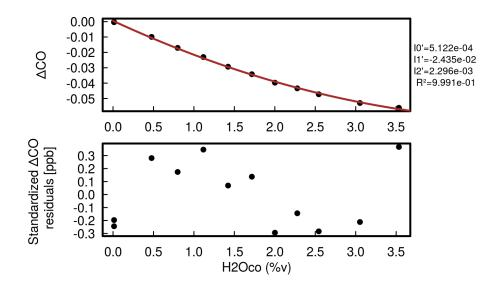
$H_2O$  correction coefficients determined by ATC
