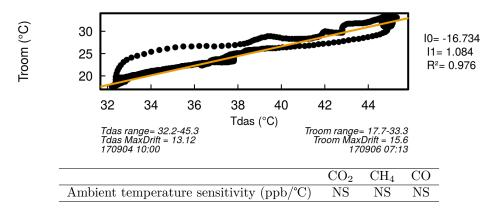
Not significant (NS) if R<sup>2</sup><0.45 or the absolute value of the slope lower than 5, 0.1 and 0.2 ppb/°C for CO<sub>2</sub>, CH<sub>4</sub> and CO respectively
