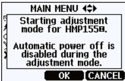
4. Select **OK** to move on to the adjustment and select the quantity you want to adjust. The list of quantities varies depending on the configuration of your HMP155.
