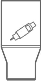
4. Loosen the screw of the sensor clamp with your fingers and insert the HMP155 probe in the larger outer hole at the bottom of the radiation shield.
