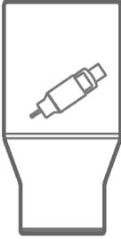
5. Loosen the screw of the sensor clamp with your fingers and insert the HMP155 probe in the larger outer hole at the bottom of the radiation shield.
