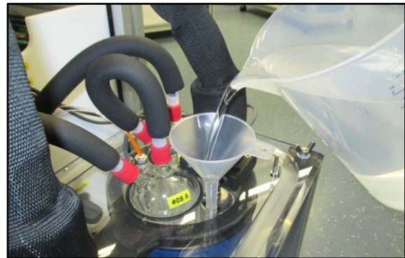
Figure 10: filling in cooling medium
